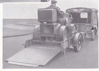
A screw-operated retractable jockey wheel at the forward end of the trailer facilitates man-handling and also aligns the coupling for attachment to the towing vehicle.
