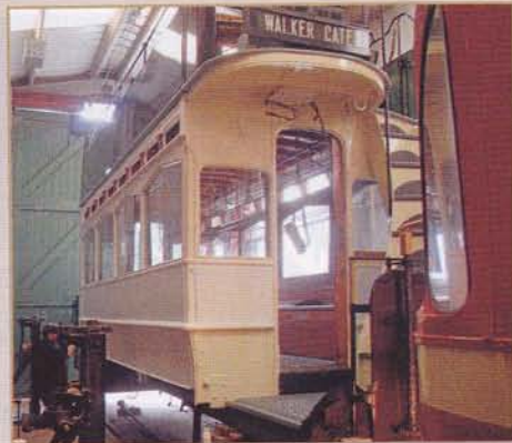
This view shows 114 lifted clear of its truck and in primer awaiting application of the new colour scheme.
