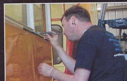
Phil picks out the beading below the windows on 114. Such work transforms the appearance but is extremely time consuming!
