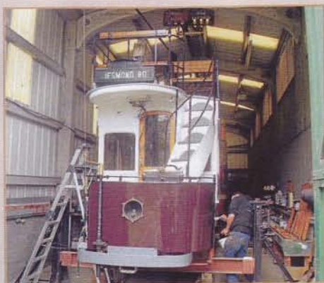
114 being repainted, with the dash panels having received their first coats of colour.
