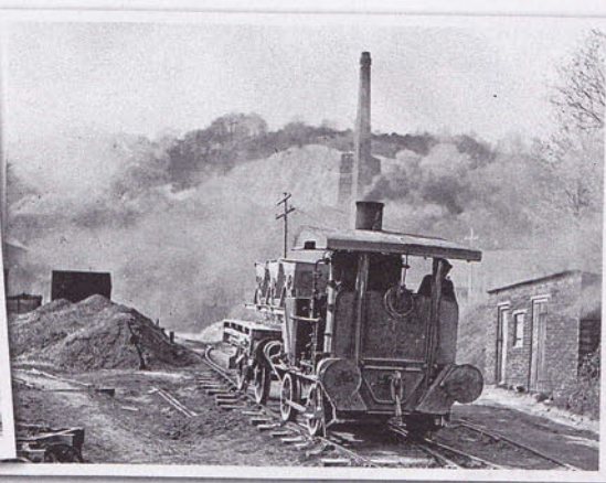
Far left: Running with its 4th boiler in the 1940s, note cab roof and substantial end supports to stabilise the tall boiler.
