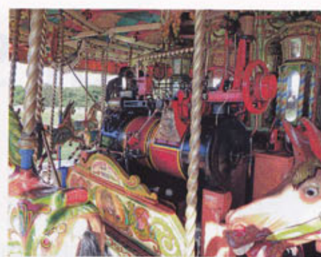
Powering the Gallopers is Savage centre engine No 627 of 1895 May Queen , restored after arriving at Beamish and steamed for the first time since the 1940s. The organ was also completely restored. TERRY PINNEGAR
