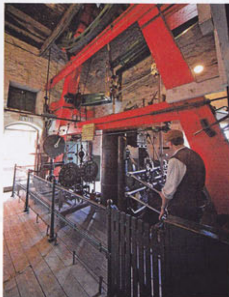
The engine most frequently to be found in steam is this 1855 Crowther of Newcastle vertical winding engine, originally sited at Beamish No 2 pit, which closed in 1962. BEAMISH
