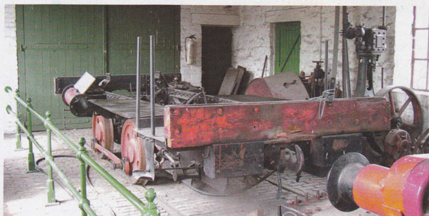
Above and left: No. 18 today: The rolling chassis is on display in the colliery engine shed at Beamish. Some repairs have been made to the frames and the rear axle has been replaced. However, the boiler - a new item built by H.A. McEwen in 1997 - is outside. It requires a small amount of work before the engine can steam. The remains of the original boiler can be seen on the right. BEAMISH.
