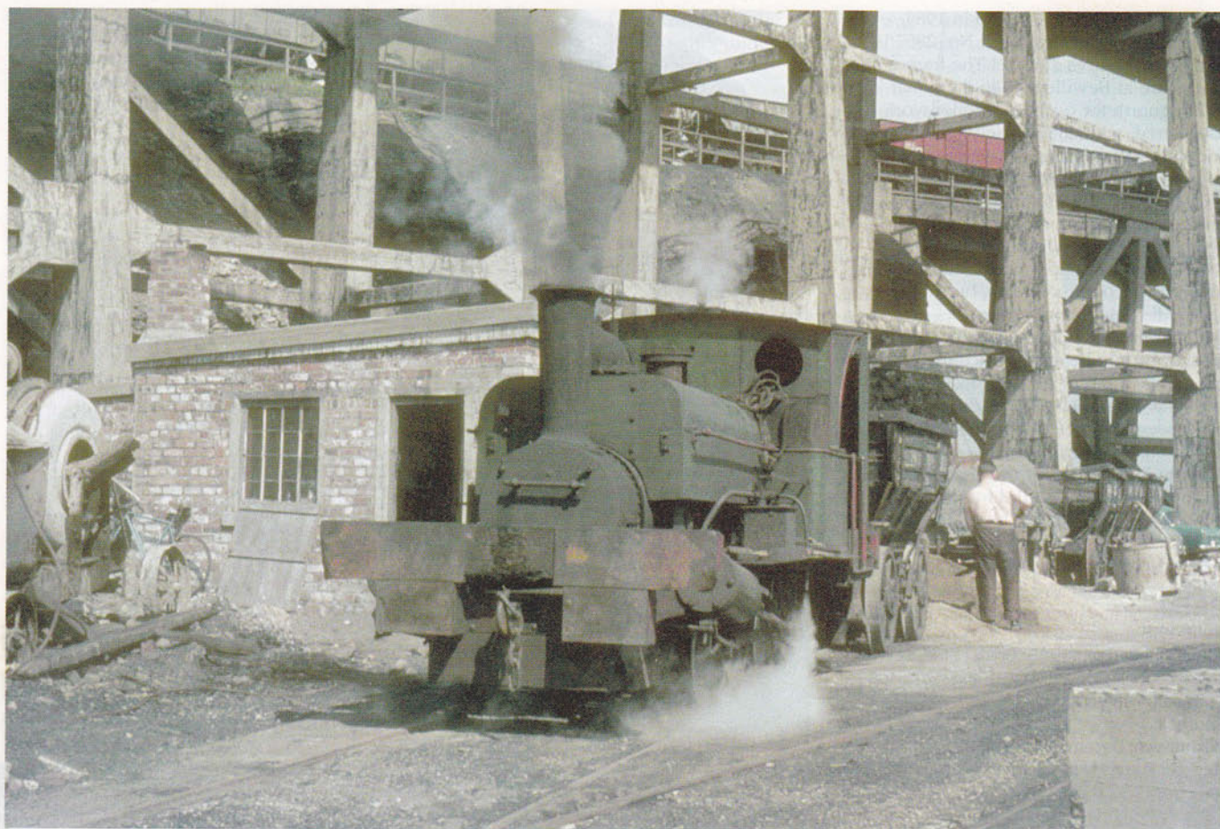
Above: The most unlikely celebrity steam locomotive? Seaham Harbour Dock Company No. 18 shunts a chaldron wagon under the staithes at Seaham Harbour in 1963. The locomotive's five-foot wheelbase led to its continued survival on the tight curves and lightly laid track on the quayside. TONY BOWLES/ RESTORATION & ARCHIVING TRUST.
