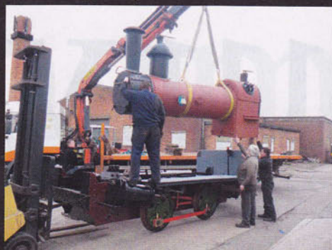
After rebuilding in Derbyshire, the boiler returns.
