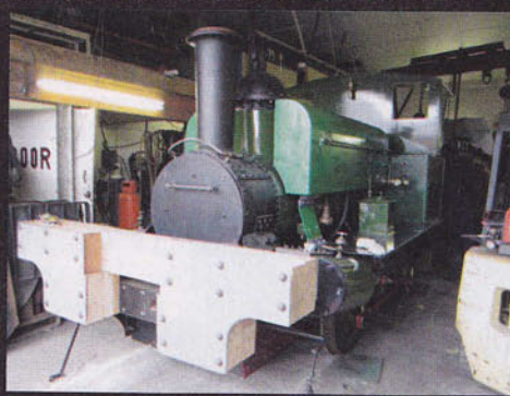
Nearly there. No. 18 complete with new wooden buffers.
