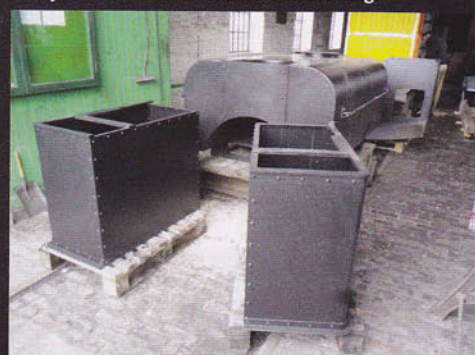
Newly fabricated tank and bunkers await fitting.
