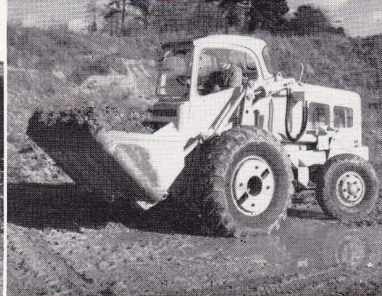
The '800' TC A front wheel drive shovel with a forward position for the operator and torque convertor transmission. The side arm arrangement is similar to the '700'.
