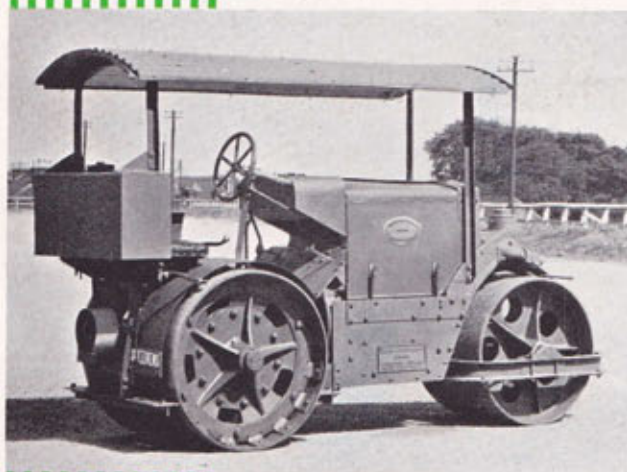
CENTRE A COLONIAL MODEL WITH AWNING, WATER SPRAYERS AND POWER TAKE-OFF (DRIVING PULLEY)
