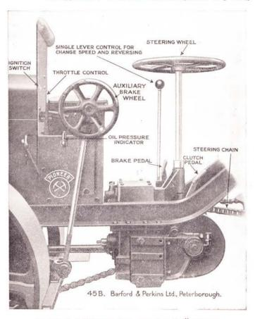
CONTROLS, GEAR BOX, ETC., OF TYPE "B" ROLLER.
