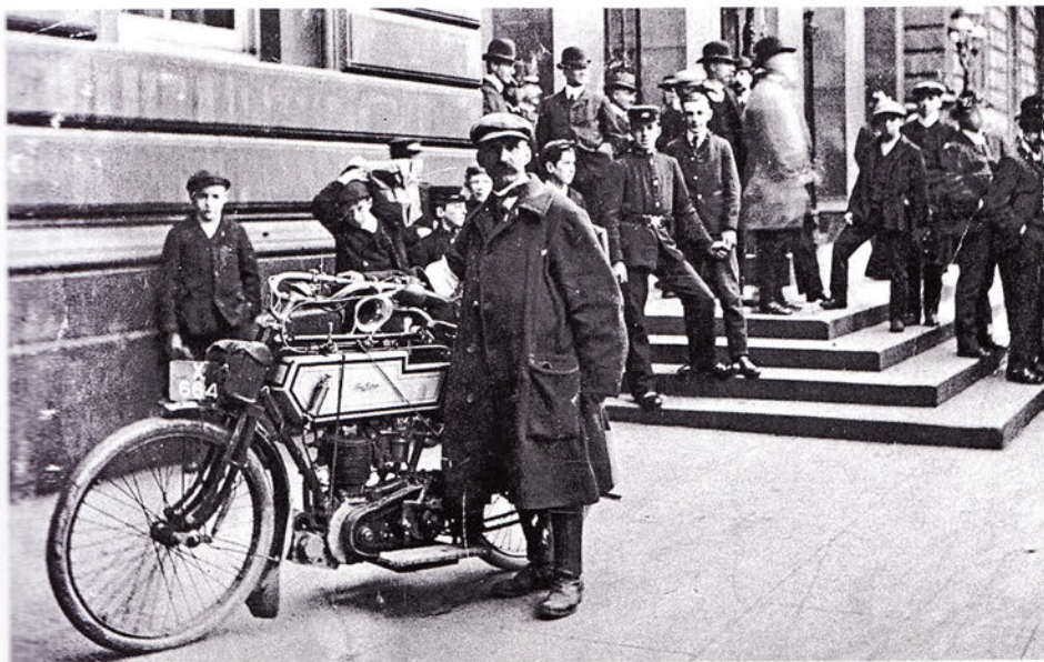
Jimmy Moore in 1906 outside the main Post Office in Edinburgh at the completion of a long distance trial. The machine is an all chain drive 1906 Dene which is of great technical interest. It has the epicyclic gearbox which he designed and manufactured himself.
