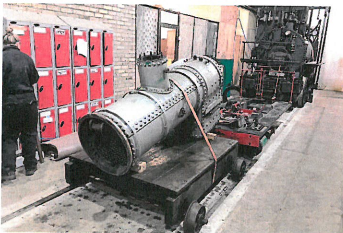
Following dismantling at the rear of the museum's tram depot, No. 721's boiler was mounted onto a trolley in readiness for its tubes to be removed. PAUL JARMAN/BEAMISH MUSEUM
