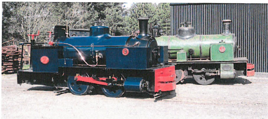
Esmé and Jack , referred to in the text, at Beamish's April 2013 Great North Steam Fair. Jack has enlarged side tanks and bunkers fitted, to make it more suitable for railway running rather than operation within the confines of a gas works. PAUL JARMAN/BEAMISH MUSEUM
