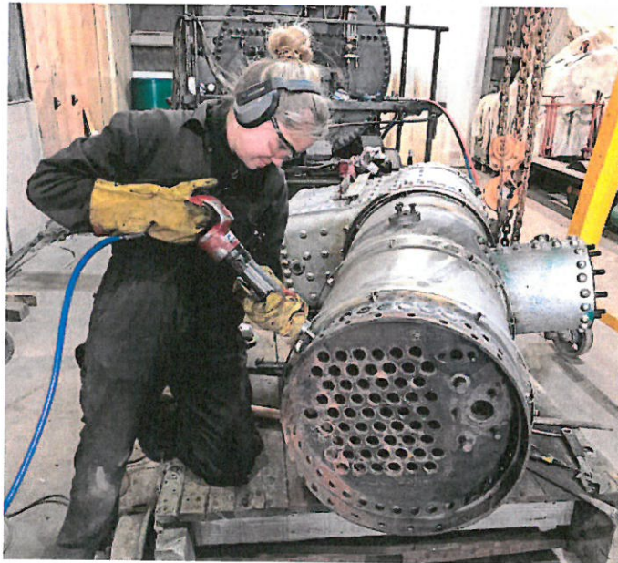
Matthew Ellis and Zoe Hart remove the front tubeplate rivets. PAUL JARMAN/BEAMISH MUSEUM
