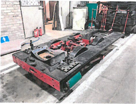
The rolling chassis of No. 721 will be moved into the museum's machine shop once the boiler has been prepared for repair. The well tank (beneath the smokebox saddle) will be removed for repair, which may entail removal of the cylinders too. PAUL JARMAN/BEAMISH MUSEUM
