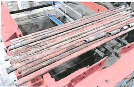
The original brass tubes fitted to No. 721's 1944 Hunslet-built boiler. They remain in excellent condition, though will be replaced with steel tubes when the boiler is reassembled. PAUL JARMAN/BEAMISH MUSEUM
