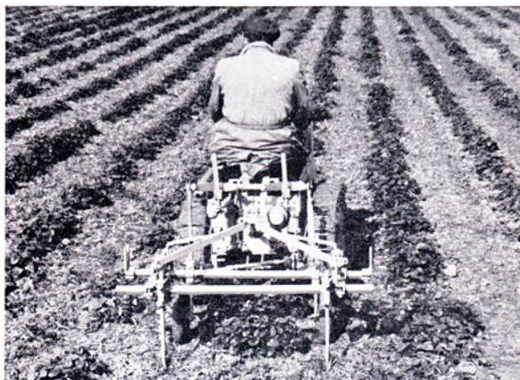
C67 toolbar fitted with sweeps
