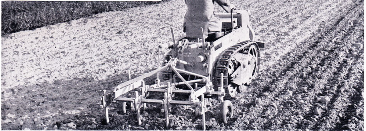
C67 toolbar working with tractor fitted with hydraulic lift
